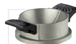
Concave block adapter for 1 L round flasks P/N 504-94000-00
